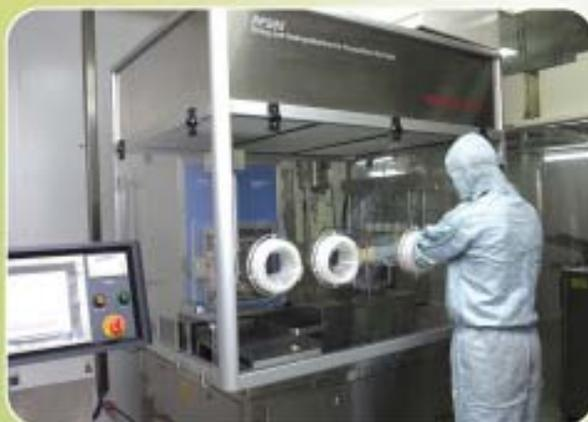
Filling & Sealing machine for pre-filled syringe
