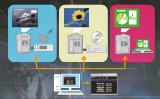
Use your computer's Web browser to fully control multiple EMP-8300 projectors connected to the network. Make settings for various functions, and access the projector's menu items and functions found on the remote control.
