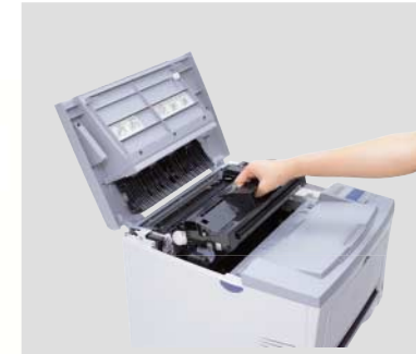
Imaging cartridge easily assessed and replaced
